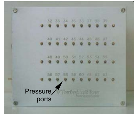
A 32-channel DP module showing the pressure ports on the top surface
