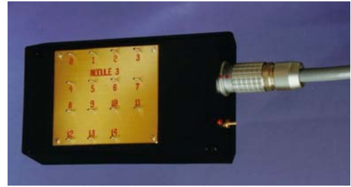
Lightweight 15-channel DP module, with the 16 th channel used for a temperature sensor
